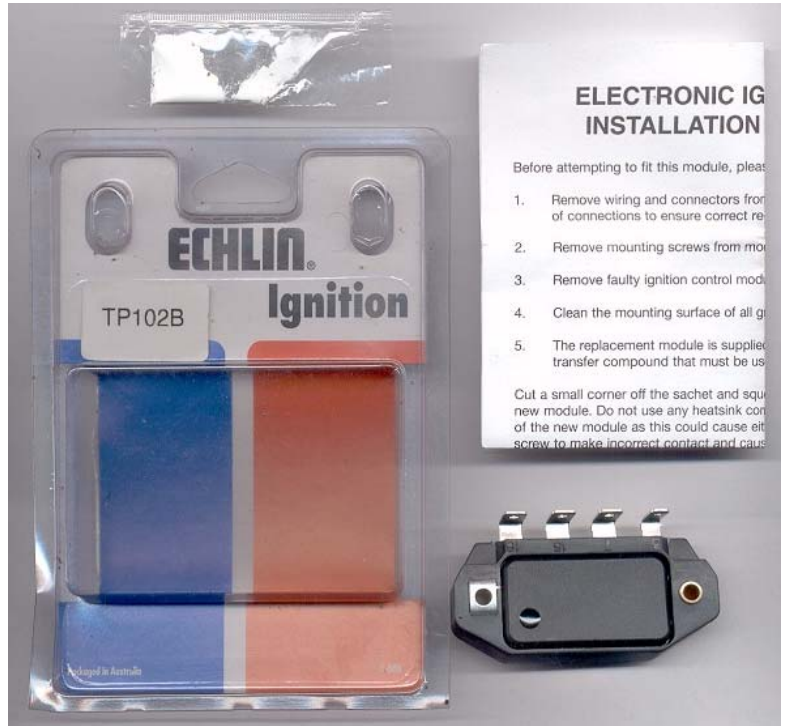
The replacement ECHLIN modules
